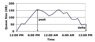
Figure 5. *The size of bfr's buffer over time.* While the queue size increases during the day, it decreases during night when there is less traffic. At the end of this particular day, Bunker's offline component still had 50GB of unprocessed raw trace left in the buffer.
