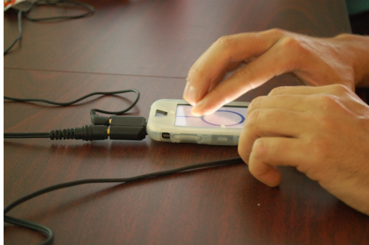
Figure 5.5: Participant using the Timbremap device during a study. The shape is shown on the device screen for experimenter reference. This particular participant is completely blind and could not see the shape. A Y-splitter was used in the audio jack to enable the experimenters to also hear the sonification given to the participant.
