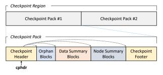
Figure 2: Each F2FS checkpoint pack contains a header followed by a variable number of orphan blocks.
