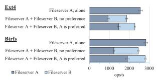
Figure 6: Throughput of prioritized caching over LRU caching with one or two file servers for Ext4 and Btrfs.
