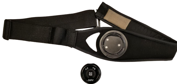
Figure 2.4: Zephyr BioHarness 3.0 used as a ground truth respiratory rate monitor.
